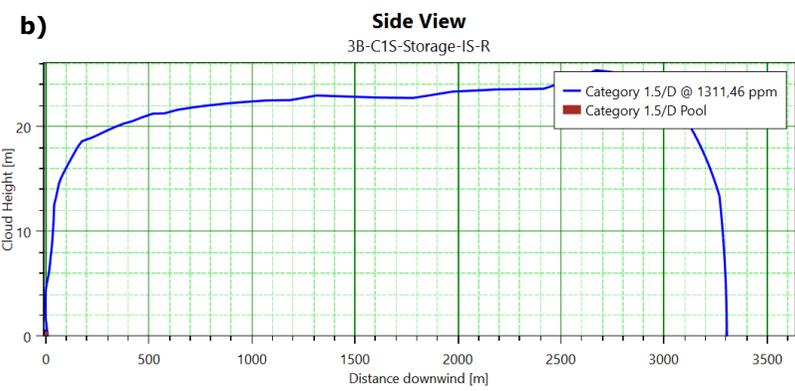
**Figure 7-6 Concept 1, Segment 3 – storage tank, liquid release from the tank inlet line on the land, rupture release scenario. View time is 1650 seconds @ toxic concentration of 1311,46 ppm (0.1% fatality) @ 1.5D wind conditions; (a) toxic cloud footprint (view from above), i.e. cloud width, m vs cloud downwind distance, m, (b) cloud sideview, i.e. cloud height, m vs cloud downwind distance, m. Dispersion surface – open water.**
