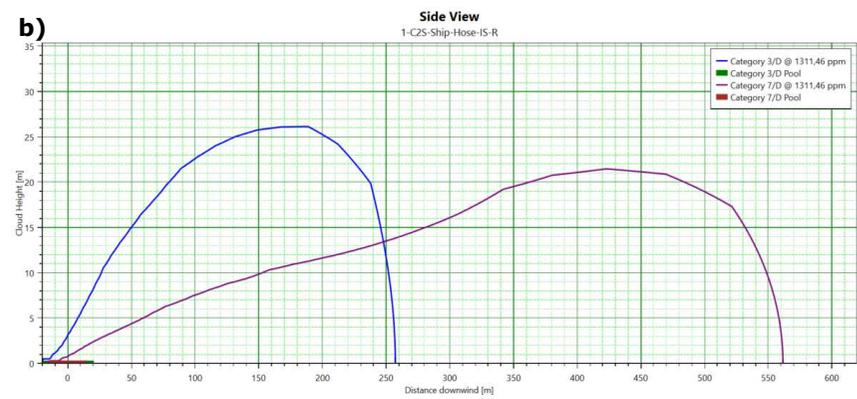
**Figure 7-8 Concept 2, Segment 1 – ship transfer by hose, cold ammonia spill to water, rupture release scenario. View time is 190 seconds @ toxic concentration of 1311,46 ppm (0.1% fatality) @ 3D & 7D wind conditions; (a) toxic cloud footprint (view from above), i.e. cloud width, m vs cloud downwind distance, m, (b) cloud sideview, i.e. cloud height, m vs cloud downwind distance, m Dispersion surface – open water.**
