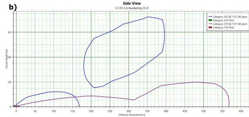
**Figure 7-7 Concept 1, Segment 5 – loading arm, pressurized ammonia spill to water, rupture release scenario. View time is above 100 seconds @ toxic concentration of 1311,46 ppm (0.1% fatality) @ 1.5D wind conditions; (a) toxic cloud footprint (view from above), i.e. cloud width, m vs cloud downwind distance, m, (b) cloud sideview, i.e. cloud height, m vs cloud downwind distance, m. Dispersion surface – open water.**
