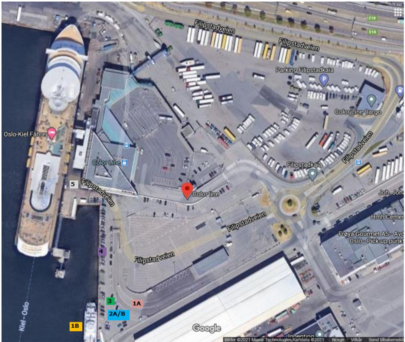
**1A** - Ammonia transfer from the truck; **1B** - Ammonia transfer from the ship; **2** - Receiving manifold; **3** - Storage tank; **4** - Process pipe; **5** - Loading Arm
