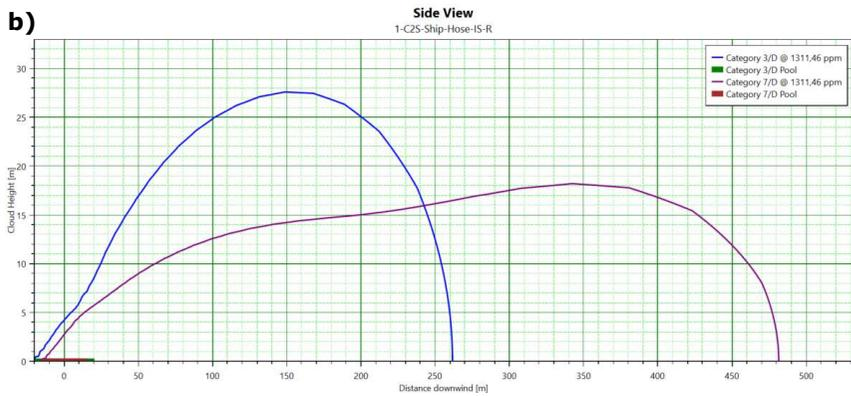
**Figure 7-5 Concept 1B/2, Segment 1B/1 – ship transfer by hose, cold ammonia spill to water, rupture release scenario. View time is 190 seconds @ toxic concentration of 1311,46 ppm (0.1% fatality) @ 3D & 7D wind conditions; (a) toxic cloud footprint (view from above), i.e. cloud width, m vs cloud downwind distance, m, (b) cloud sideview, i.e. cloud height, m vs cloud downwind distance, m Dispersion surface – land.**
