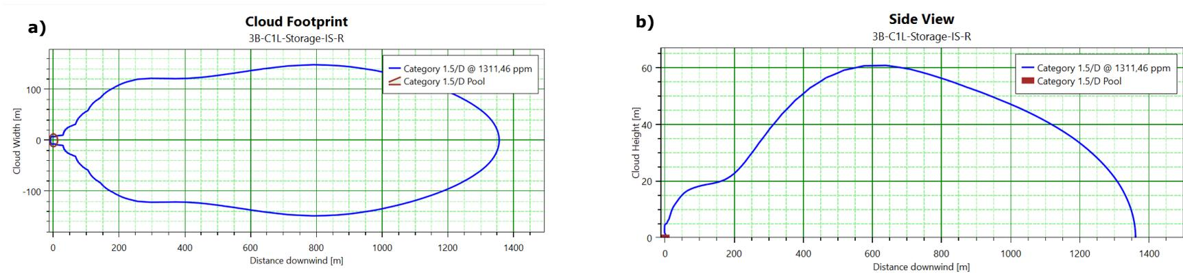
**Figure 7-3 Concept 1, Segment 3B – storage tank, liquid release from the tank inlet line connection on land, rupture release scenario. View time is 1650 seconds @ toxic concentration of 1311,46 ppm (0.1% fatality) @ 1.5D wind conditions; (a) toxic cloud footprint (view from above), i.e. cloud width, m vs cloud downwind distance, m, (b) cloud sideview, i.e. cloud height, m vs cloud downwind distance, m. Dispersion surface – land.**
