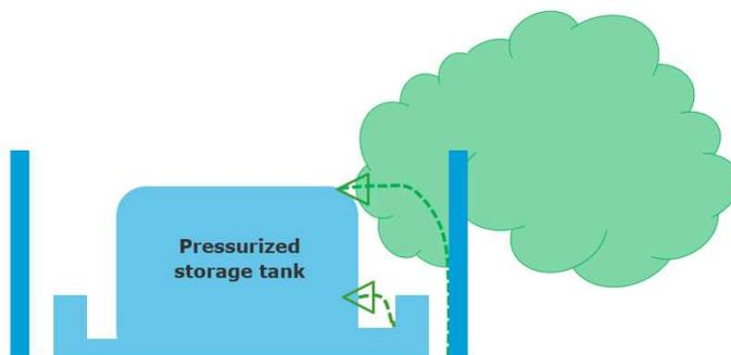
**Figure 4-5 Release from the storage tank's inlet and outlet external connections with release being obstructed by the bund and a wall structure followed by rainout inside the bund/wall**
