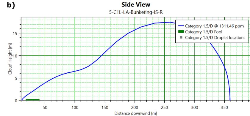
**Figure 7-4 Concept 1, Segment 5 – loading arm, pressurized ammonia release on land, rupture release scenario. View time is above 200 seconds @ toxic concentration of 1311,46 ppm (0.1% fatality) @ 1.5D wind conditions; (a) toxic cloud footprint (view from above), i.e. cloud width, m vs cloud downwind distance, m, (b) cloud sideview, i.e. cloud height, m vs cloud downwind distance, m. Dispersion surface – land.**
