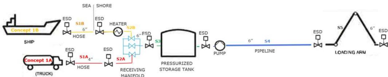
**Figure 4-1 Process flow diagram Concept 1A-bunkering of ammonia by trucks; Concept 1B-bunkering of ammonia by ship**
