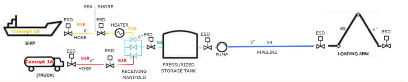
**Figure 2-2 Simplified process flow diagram Concept 1**
