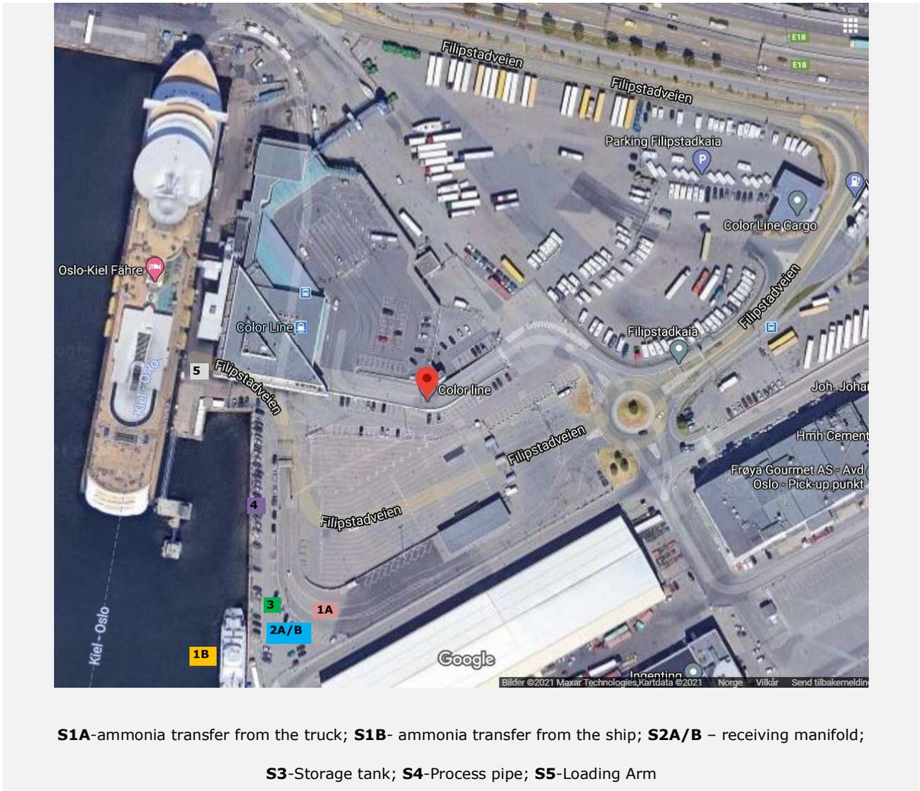
**S1A**-ammonia transfer from the truck; **S1B**- ammonia transfer from the ship; **S2A/B** – receiving manifold;
