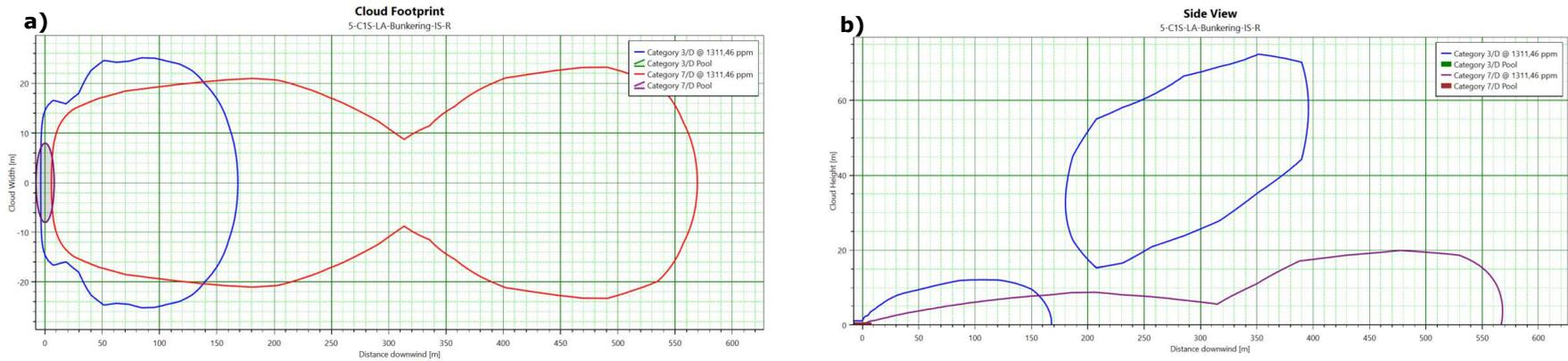
**Figure 7-7 Concept 1, Segment 5 – loading arm, pressurized ammonia spill to water, rupture release scenario. View time is above 100 seconds @ toxic concentration of 1311,46 ppm (0.1% fatality) @ 1.5D wind conditions; (a) toxic cloud footprint (view from above), i.e. cloud width, m vs cloud downwind distance, m, (b) cloud sideview, i.e. cloud height, m vs cloud downwind distance, m. Dispersion surface – open water.**
