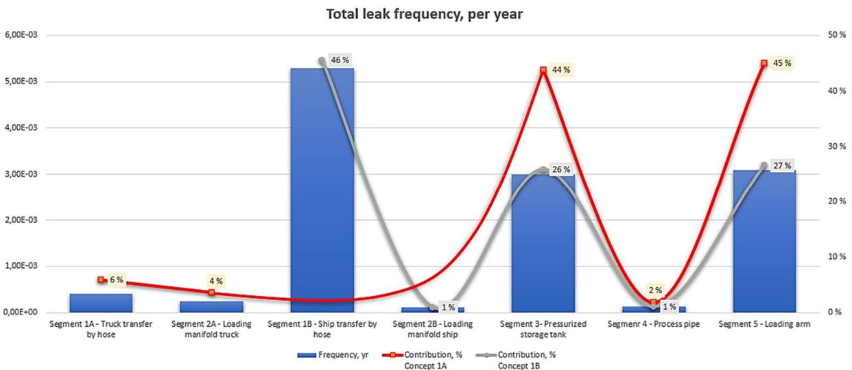
**Figure 7-1 Total annual leak frequency and % contribution, Concepts 1A and 1B**
