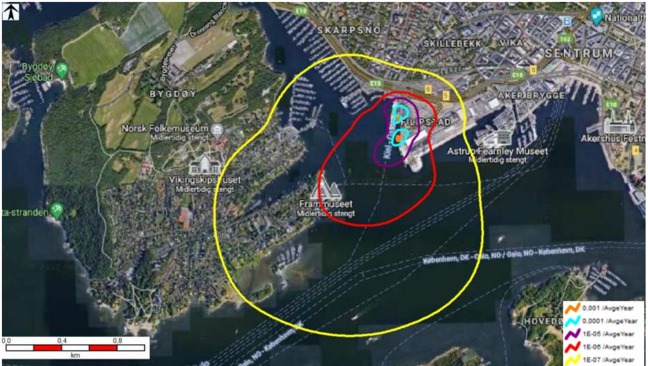
**Figure 7-13 LSIR contour – Concept 1B**
