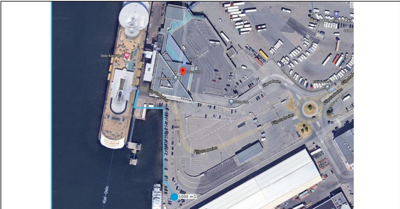
**Figure 2-1 Ammonia bunkering facility, from storage tank via process pipe to the passenger ship (shown in blue line).**
