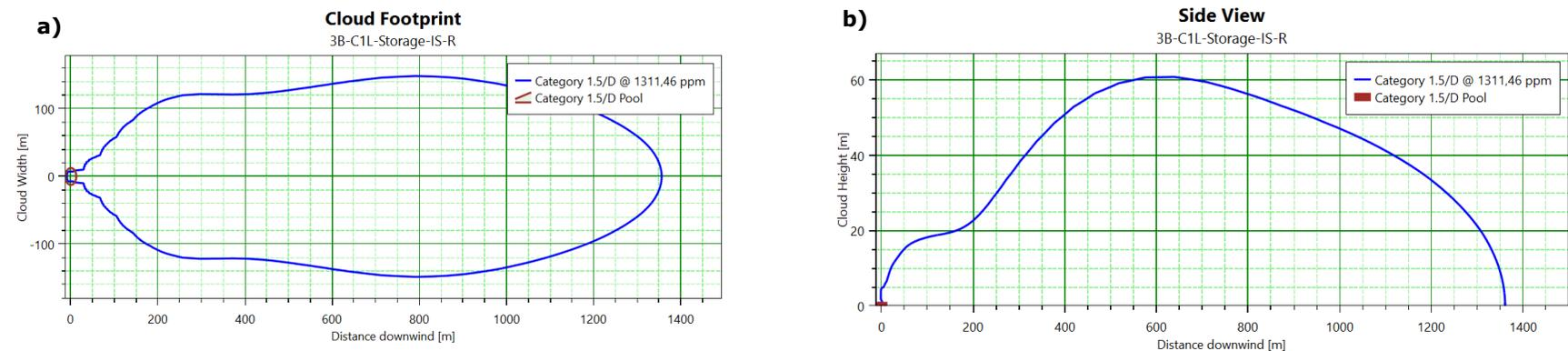
**Figure 7-3 Concept 1, Segment 3B – storage tank, liquid release from the tank inlet line connection on land, rupture release scenario. View time is 1650 seconds @ toxic concentration of 1311,46 ppm (0.1% fatality) @ 1.5D wind conditions; (a) toxic cloud footprint (view from above), i.e. cloud width, m vs cloud downwind distance, m, (b) cloud sideview, i.e. cloud height, m vs cloud downwind distance, m. Dispersion surface – land.**
