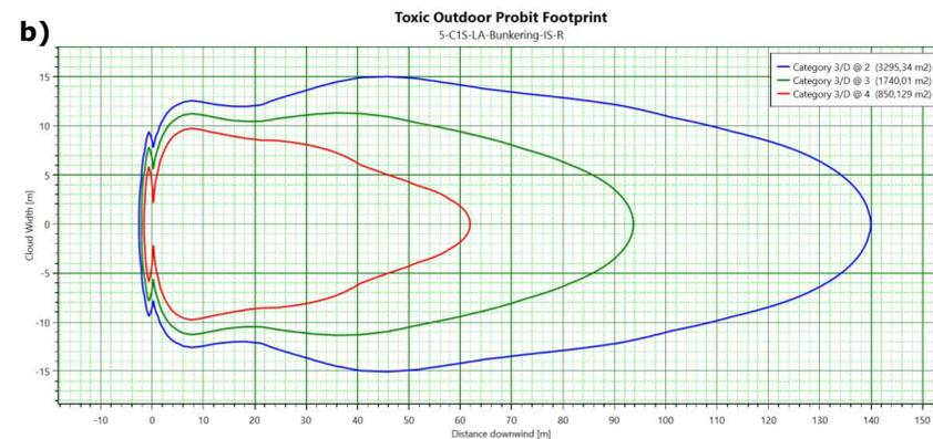
**Figure 7-10 Concept 1, Segment 5 – loading arm, rupture release scenario; (a) dispersion surface – land @ 1.5D wind conditions, (b) dispersion surface – open water @ 3D wind conditions.**
