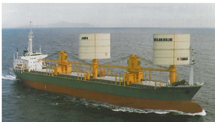
Figure 7: The first deep sea merchant ship designed and outset for sail-assisted propulsion, a 26000 dwt bulk/log carrier Usuki Pioneer (Brett, 1984).
